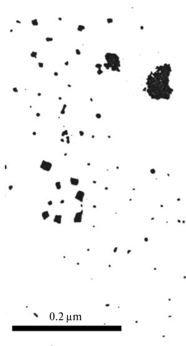
Fig. 1. Electron micrographs of CsI particles and aggregates deposited on a collector; T_g = 313 K, t = 10 s, H = 5 cm, a JEM-100B electron microscope.
